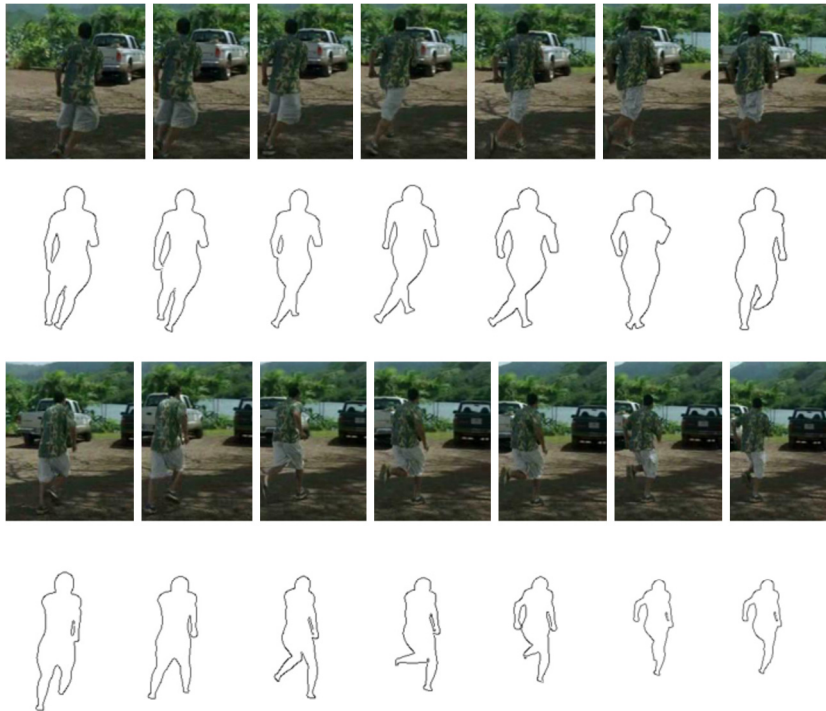
Fig. 1. Illustration of video frames and their corresponding silhouette boundary curves. The silhouette boundary curves of the moving human subject are extracted from each frame using a modified Mask R-CNN (He et al., 2017), which only detects human subjects.
